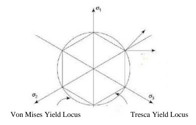
Fig 1: Locus of Tresca and Von Mises yield criteria on Deviatoric Plane
